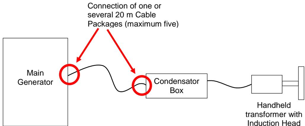
The connections are the same on the main-generator, the condensator box and between each of the hose packages. The pictures below show the connections consisting of two water connections and one electrical contact:
