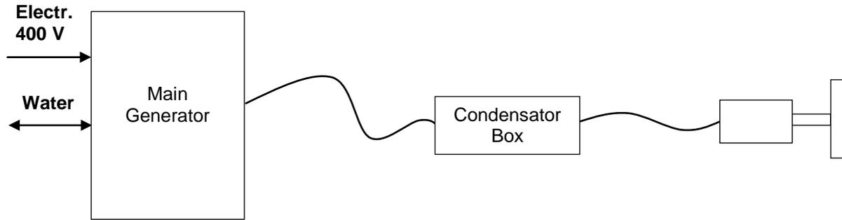
**IMPORTANT! Do not connect the electricity or water supply to the RPR-1650 until you have completed assembly of all cable packages between the main generator and the condensator box and the induction head.**
