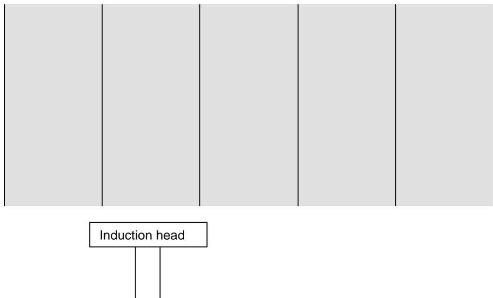
When you remove the coating (See section [7 Removal of paint and coatings, page 17](#)), you drag the induction head over each second marked-up field. This prevents the overheating on the edges. Then go back and take the other marked-up fields when the steel temperature has returned to normal.
